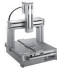
Type Gate, 3-axis Stroke X-axis: 200 mm / Y-axis: 200 mm / Z-axis: 50mm / 100mm Load capacity X-axis: 10kg / Z-axis: 2kg
