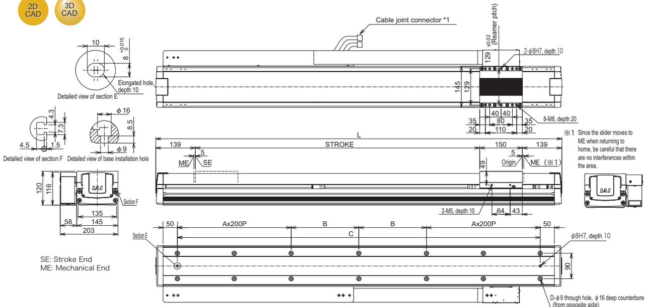
Note: Due to their structure, models with a mid-support cannot be positioned horizontally on their side or vertically.
