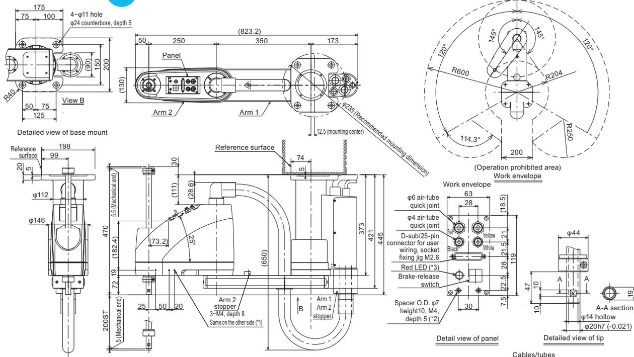
\*1: The prepared hole 3-M4, depth 8 passes through the side panel of the arm. If the mounting screw is long, make sure it does not contact internal components.
