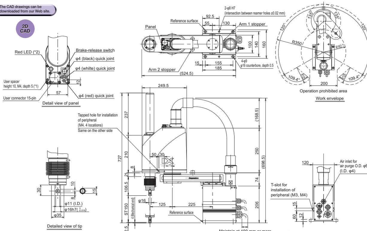
\*1: The external force applied to a spacer must not exceed 30 N in the axial direction, or 2 N·m in the rotating direction. (for each spacer)
