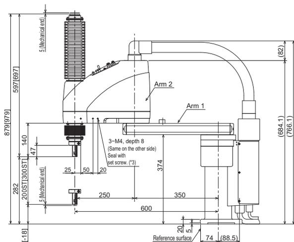
The values within □ indicate the specifications for axis 3 (vertical axis) 300 mm.
