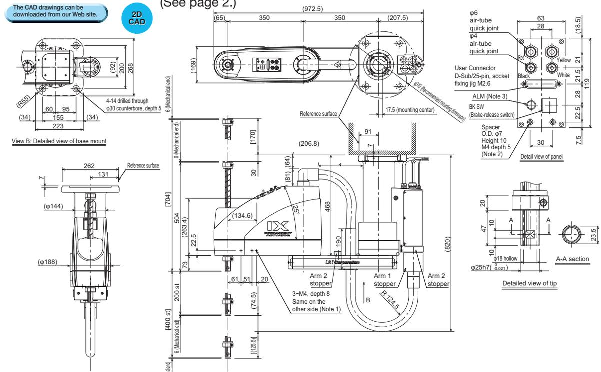
Note 1: The bottom hole 3-M4, depth 8 passes through the side panel of the arm.
