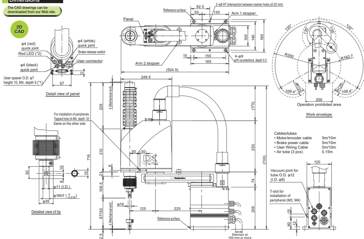
\*1: The external force applied to a spacer must not exceed 30 N in the axial direction, or 2 N·m in the rotating direction. (for each spacer)
