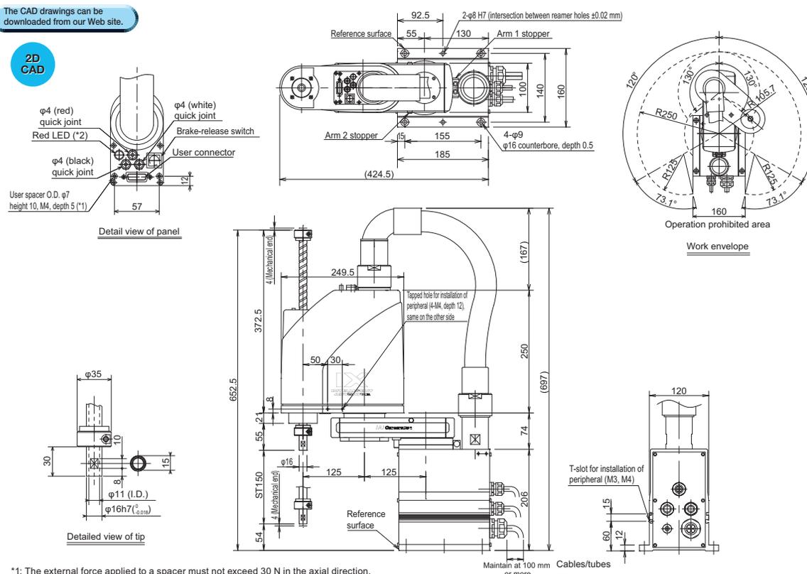
\*1: The external force applied to a spacer must not exceed 30 N in the axial direction, or 2 N·m in the rotating direction. (for each spacer)
