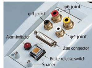
\*1 24 V DC power must be supplied regardless of whether or not the brake-release switch is used.
