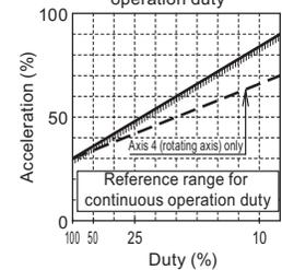
IX500 standard Reference acceleration/deceleration settings for CP operation
