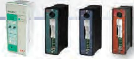
Unlike conventional controllers, the PMEC/PSEP/ASEP/DSEP require only a few movement positions. These 230 VAC MEC ("Mechanical Engineer Control") and 24 VDC SEP ("Simple Easy Positioner") controllers are for applications where the actuator only travels between 2 or 3 points, which is usually the case with air cylinders.
