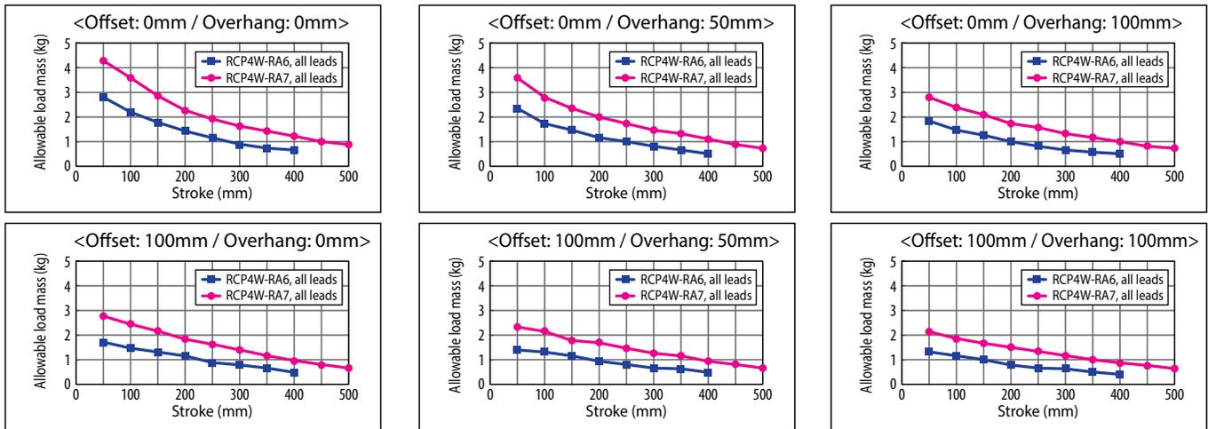
Allowable load calculation conditions: Load mass corresponding to a guide traveling life of 5,000 km, considering moments generated by acceleration/deceleration. (Acceleration: 1 G / Speed: 500 mm/s)
