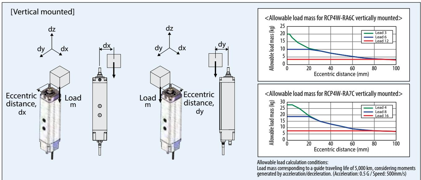
Allowable load calculation conditions: Load mass corresponding to a guide traveling life of 5,000 km, considering moments generated by acceleration/deceleration. (Acceleration: 0.5 G / Speed: 500mm/s)
