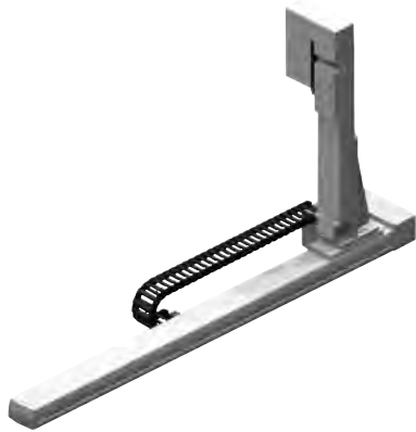
Wiring 1 with cable track
