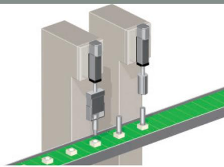
ROBO Cylinders are used in press-fitting and assembly of plastic parts. Assembly is done using positioning, and press-fitting is done using a push motion operation.
