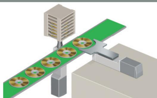
ROBO Cylinders are used to raise and lower stockers in a pitch feed operation. ROBO Cylinders use the acceleration/deceleration function for inserting stocker discs.
