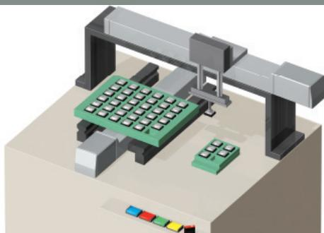
ROBO Cylinder is used on the X axis and Y axis. This is a low-cost pick & place unit.
