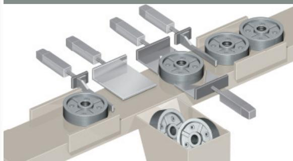
Multiple ROBO Cylinder axes are used in a screw inspection line, to help with positioning work pieces, positioning during inspection, and sorting defective parts. The controller uses XSEL5, and one controller can control all axes.
