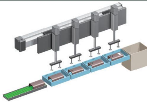
A ROBO Cylinder is used to move works to vertical positions on a transfer device to various processes to provide a compact line.
