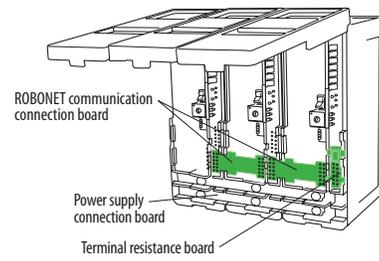
(connected part in ROBONET unit)
