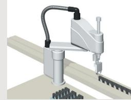
Example) Palletization of work part using SCARA robot
