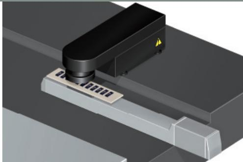
ROBO Cylinder's pitch feed mode is used to feed work pieces in a leather marking process.
