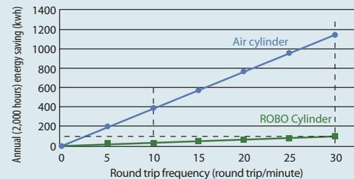
**The ROBO Cylinder is already highly energy efficient in comparison to air cylinders
