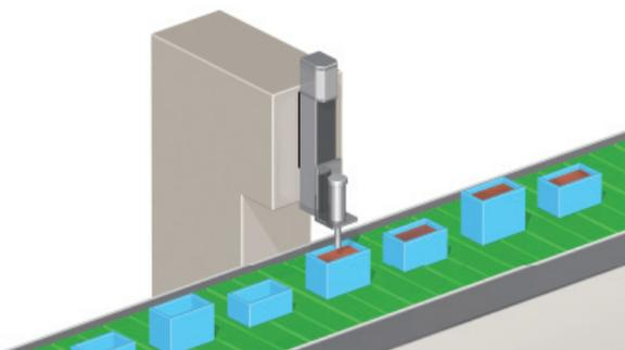
ROBO Cylinders are used to fill containers at different heights. Control of multiple positions makes it possible to handle many item types.
