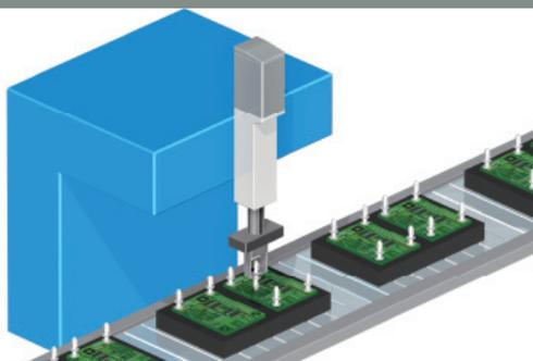
The push motion operation of the ROBO Cylinder is used to insert spacers in printed circuit boards.
