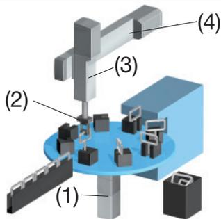
All operations including horizontal/vertical movement, gripping and rotation are performed with ROBO Cylinders alone. Connecting the controller to a field network also makes it possible to reduce wiring.
