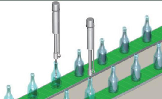
This device raises and lowers a nozzle that is inserted into a shampoo container while it inserts shampoo. This uses pulse train control to adjust speed.
