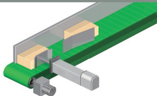
Work pieces are pushed against the wall using the push motion operation, and then aligned.
